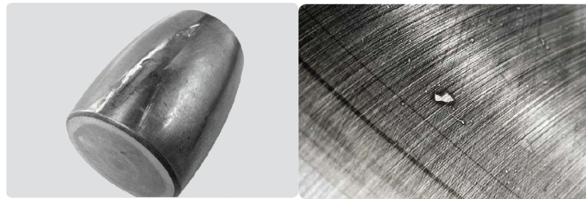
Figure 7. Plastic deformation failure. Overload ( left ) and indentation ( right ) [27]. Courtesy of SKF.
