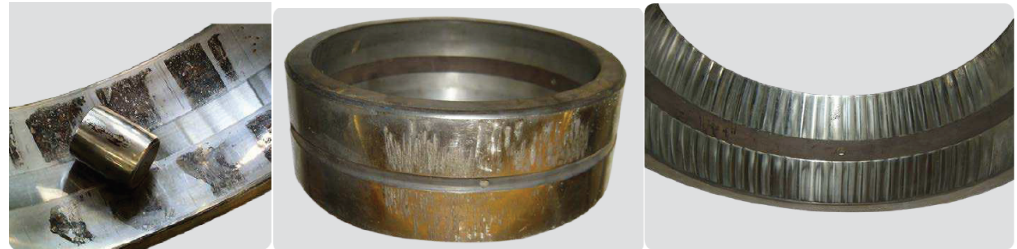
Figure 5. Corrosion failures. Moisture (left), fretting (middle), and brinelling (right) [27]. Courtesy of SKF.
