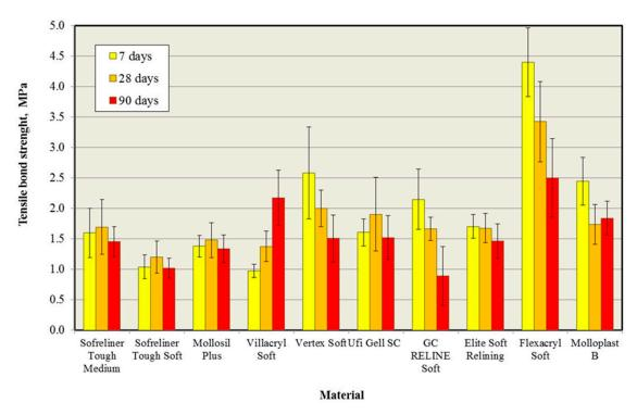
**Figure 2.** Average values of the tensile bond strength of the tested relining materials with acrylic material for denture plates during 90 days of storing in distilled water.
