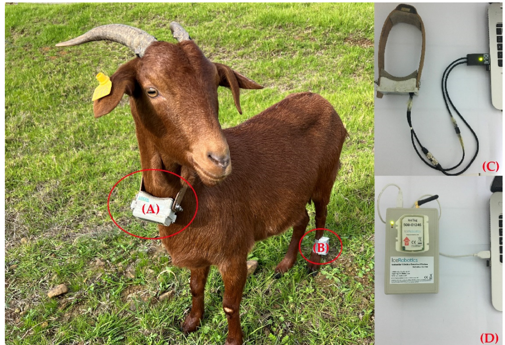
Figure 2. Indigenous goat of Beni Arouss fitted with GPS collar on the neck (A) and IceTag sensor on the rear left leg (B). Downloading GPS collar (C) and IceTag (D) data.
