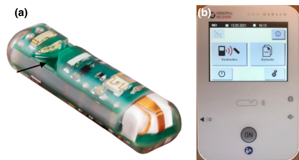
Figure 1 (a) The HemoPill capsule. Size: 7.0 mm \times 26.3 mm. The black arrow is pointing at the measuring slot for blood entry. On one slot side, light of different wavelengths is emitted by LEDs. On the other side, intensity of the light is measured. According to different absorption properties of various substances passing through the slot, a HemoPill indicator (HI) is calculated and mapped on a display of a wireless receiver. (Source: Ovesco Endoscopy AG, Tübingen, Germany). (b) The wireless HemoPill receiver for real-time data display.
