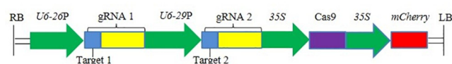
Fig 1. Schematic representation of recombinant plasmid pHDE-35S- mCherry . U6-26P and U6-29P are the promoters of two gRNAs, respectively. 35S is the promoters of Cas9, and 35S is the promoters driving of mCherry gene.
