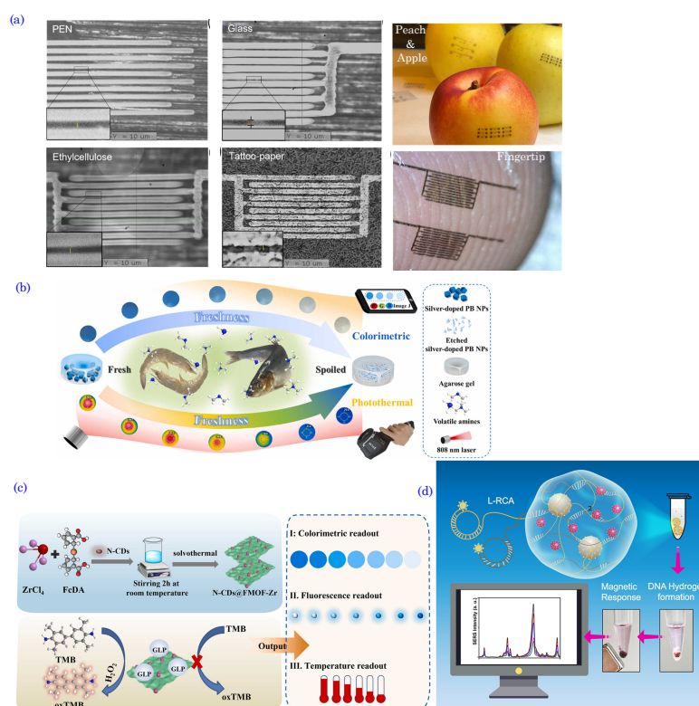
Figure 14. (a) Characterization of inkjet-printed gold electrodes on various conventional and edible substrates: Depiction of gold interdigitated electrodes inkjet-printed on diverse substrates: poly(ethylene 2,6-naphthalate) (PEN), glass, edible ethyl cellulose biopolymer (food additive E462), and edible tattoo paper. Visual representations of gold electrodes transferred onto distinct surfaces: (right top) peach, apple, and (right bottom) fingertip. Reprinted with permission from Sharova et al. [251], ©2023 The Royal Society of Chemistry. (b) Schematic representation of colorimetric and photothermal assessment of shrimp and fish freshness utilizing a portable silver-doped Prussian blue nanoparticles (SPB NPs) hydrogel, facilitated by a smartphone and handheld thermal imager. Reprinted with permission from Ding et al. [252], ©2022 Elsevier B.V. (c) Carbon dots anchoring ferrocene metal-organic framework nanosheet for multi-mode glyphosate (e.g., herbicide) sensing. Reprinted with permission from Luo et al. [253], ©2022 Elsevier B.V. (d) Schematic illustration of SERS aptasensor based on DNA hydrogel fishing network for ultrasensitive detection of antibacterial kanamycin (KANA). Reprinted with permission from Chen et al. [254], ©2022 Elsevier B.V.
