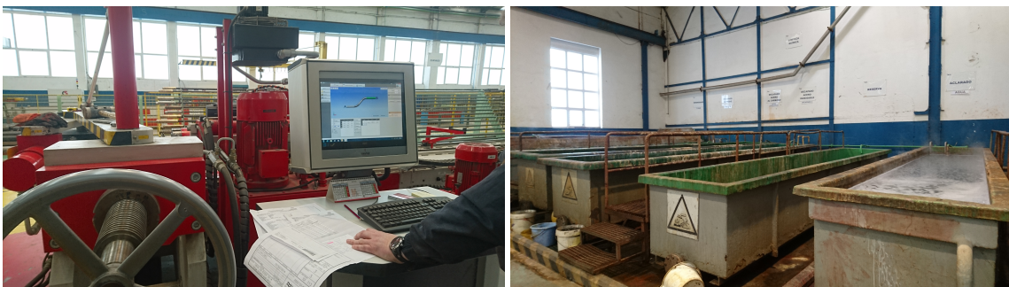
Figure 4. Computerized bending machine (left) and cleaning tubs of the pipe workshop (right).
