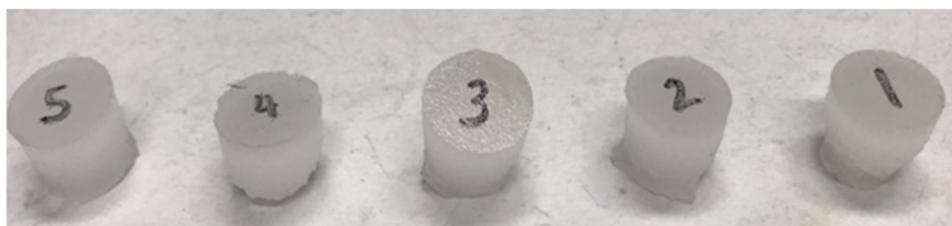
**Figure 2.** Cylindrical blend HS/PDMS 20:80 network for compression test.
