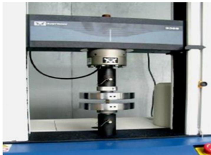
**Figure 1.** Instron universal compression-testing used for the compression test.
