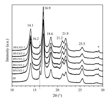
**Figure 2.** XRD patterns of PP and PP/CNT nanocomposites in the 10–30° 2θ range (\* is a peak corresponding to catalyst residue).
