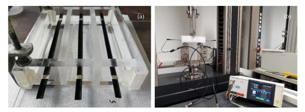
**Figure 1.** (a) Polypropylene/carbon nanotubes (PP/CNT) strips in the PMMA mold and (b) impedance measurement setup.
