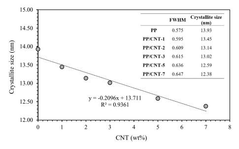
Figure 3. Crystallite size determined using Scherrer's equation for the lattice plane (110) at 14.1°.
