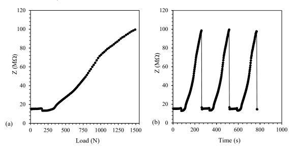
**Figure 11.** Impedance value for PP/CNT-5 nanocomposites. (**a**) Impedance (Z) variation vs. load and (**b**) load/unload cycles.
