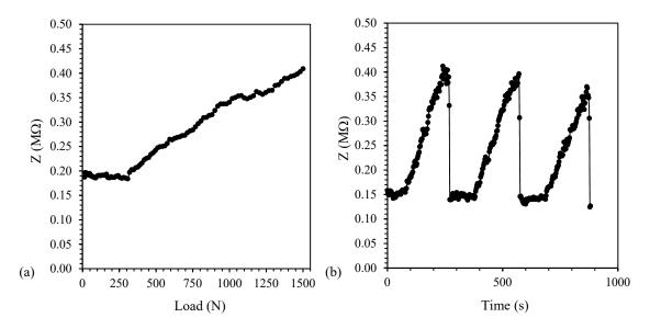
**Figure 12.** Impedance value for PP/CNT-7 nanocomposites. (**a**) Impedance (Z) variation vs. load and (**b**) load/unload cycles.
