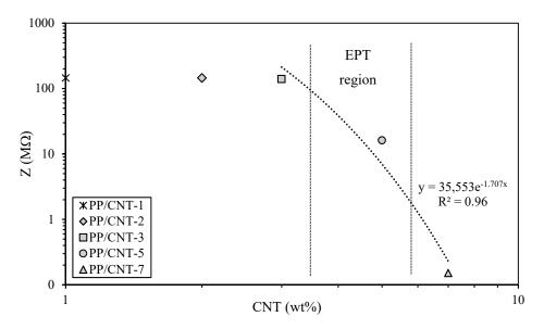
Figure 9. Impedance of the different PP/CNT nanocomposites strips.
