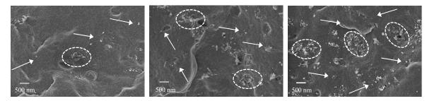
**Figure 7.** (a) PP/CNT-3, (b) PP/CNT-5 and (c) PP/CNT-7. White arrows indicate single dispersed CNTs; white ellipsis indicate CNTs agglomerates.
