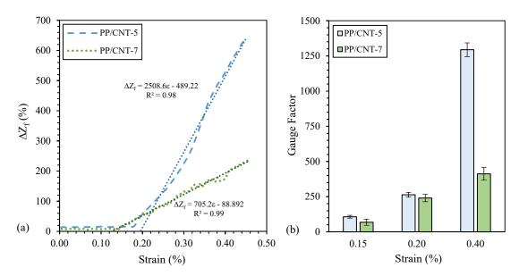
**Figure 13.** (a) fractional change in electrical impedance ( $\Delta Z_f$ ) as a function of strain and (b) Gauge Factor (GF) at fixed strains (i.e., 0.15%, 0.20% and 0.40%, respectively) for PP/CNT-5 and PP/CNT-7 nanocomposites.
