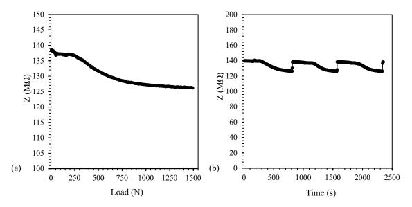
**Figure 10.** Impedance value for PP/CNT-3 nanocomposites. (**a**) Impedance (Z) variation vs. load and (**b**) load/unload cycles.
