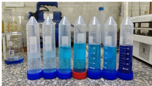
Fig. 9. Removal of MB with different concentration by the prepared geopolymer.
