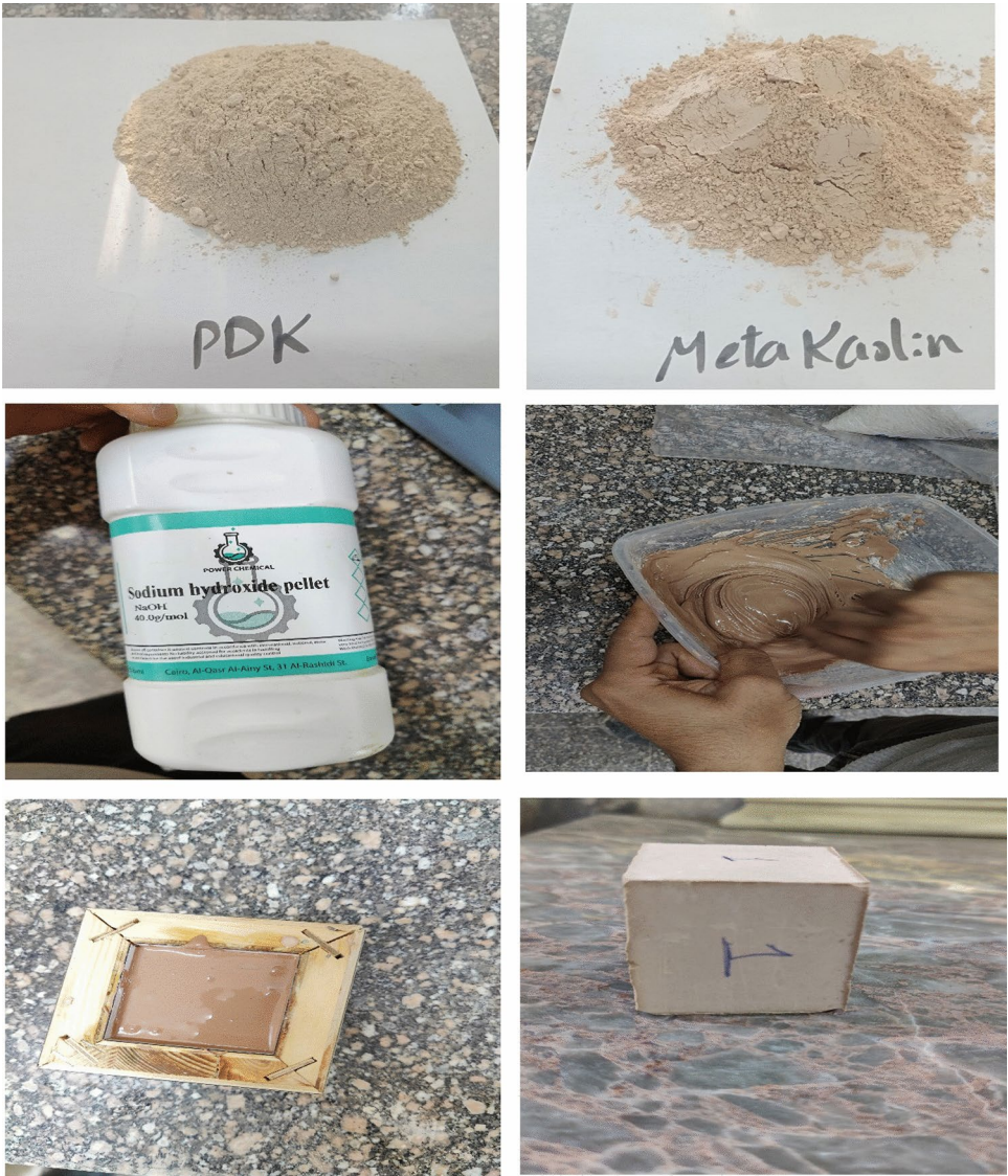
Fig. 3. Preparation of geopolymer.
