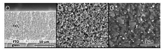
**Figure 6.** SEM images of (**a**) a photoanode cross-section, (**b**) sintered nanoparticles forming a TiO<sub>2</sub> mesoporous layer, and (**c**) platinum nanoparticles deposited on FTO counter electrode.
