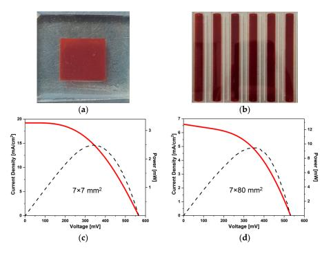
**Figure 9.** Current-voltage characteristic (red solid) and power curve (black, dashed) of  $7 \times 7 \text{ mm}^2$  (c) and  $7 \times 80 \text{ mm}^2$  (d) gel electrolyte dye-sensitized solar cell along with a photo of a small device (a) and a module (b) we created.
