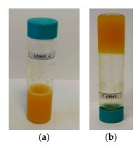
**Figure 1.** Gel electrolyte based on poly(vinylidene fluoride-co-hexafluoropropylene) and poly(dimethylsiloxane) bis(3-aminopropyl) terminated (PVDF-HFP:PDES-bAP) (9:1) before (a) and after (b) the gelation process.
