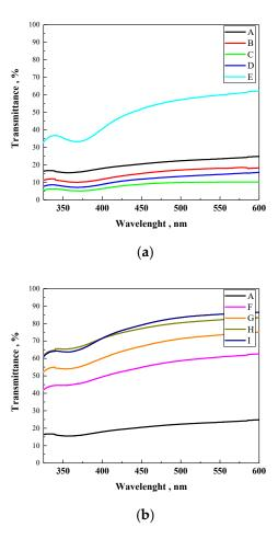
**Figure 2.** UV-Vis transmittance spectra in film for all investigated electrolytes, where **(A)** PVDF-HFP; **(B)** PVDF-HFP:PAB (9:1); **(C)** PVDF-HFP:PAB (8:2); **(D)** PVDF-HFP:PAB (7:3); **(E)** PVDF-HFP:PAB (6:4); **(F)** PVDF-HFP:PDES-bAP (9:1); **(G)** PVDF-HFP: PDES-bAP (8:2); **(H)** PVDF-HFP: PDES-bAP (7:3); **(I)** PVDF-HFP: PDES-bAP (6:4), **(a)**: A, B, C, D, E and **(b)**: A, F, G, H, I.
