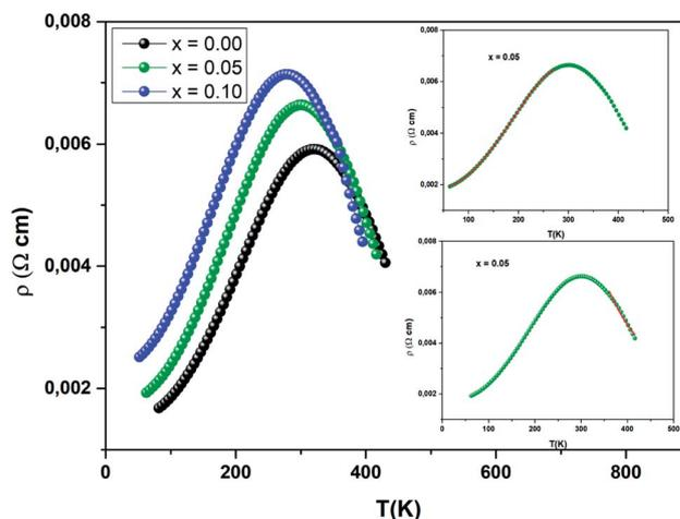
Fig. 12 Variation of  $\rho$  vs.  $T$  for three samples. The inset (top) depicts the best fit of the experimental values in the metallic region, for  $T < T_{M-SC}$ . The inset (bottom) corresponds to the fit of the data in the semi-conducting region ( $T_{M-SC} < T < T_C$ ).
