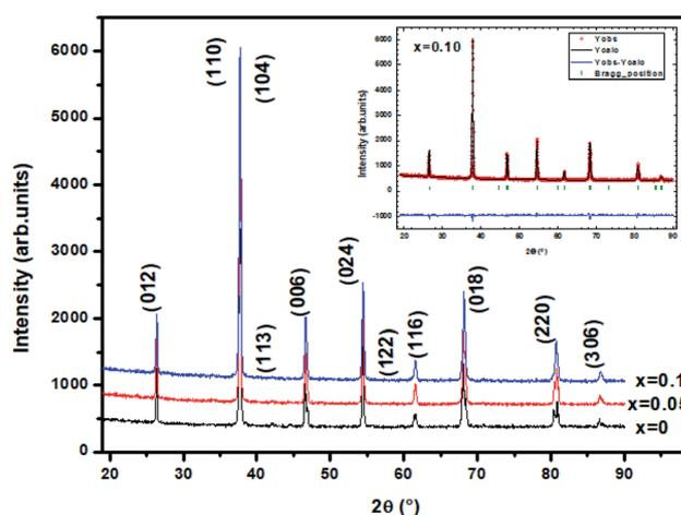
Fig. 1 XRD diagrams for solid solutions of the LBSMNO samples. Each of the peaks of these manganites are indexed in the rhombohedral structure. The inset shows the results of the Rietveld's analysis of sample  $x = 0.10$  as an example.
