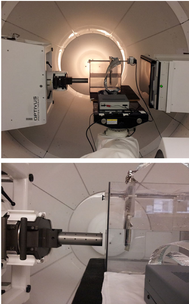
Fig. 4. DMG experimental setup for depth dose and beam profile measurements with a magnified view (bottom). Note the extended X-ray imager (top) which is used to ensure detector alignment and parallel travel with the beam central axis.
