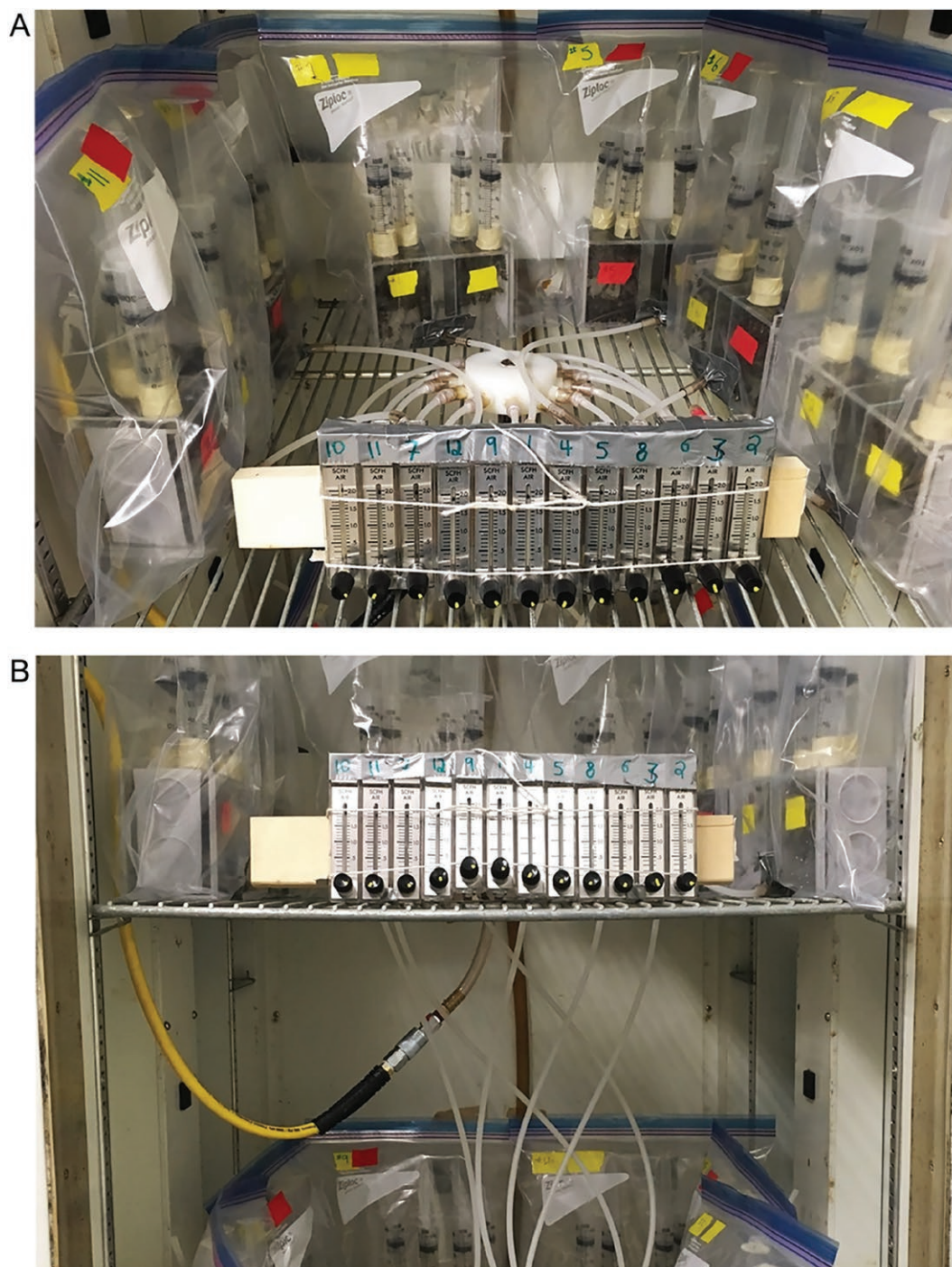
Fig. 2. Photographs of the aerosol cage study incubator setup. Showing (A) the hub splitter and individual flowmeters for each cage/bag on the two shelves, and (B) the yellow hose that supplied air from the compressor to the cages via the hub splitter.
