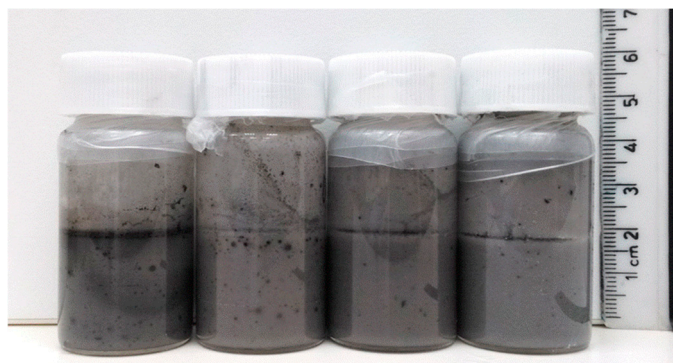
Figure 4. Toluene-in-water mixtures prepared from 2 wt% SiO 2 and 1 mg MWNTs with 0.2 M APTES and DTES. The emulsions occasionally show the presence of MWNT aggregates, as illustrated by black dots within the otherwise typically homogeneous, milky-grey mixtures. From left to right: o/w ratio = 10:90, 20:80, 30:70, 50:50.
