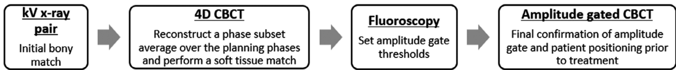
FIG. 6. The pretreatment imaging workflow used for alignment and to set the amplitude gate thresholds for treatment.
