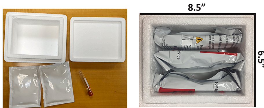
Fig. 1. (Left) Shown is the insulated packaging comprised of a 1" thick styrofoam box and 2 PCM pouches. The test tube is shown for perspective. (Right) The packaging was filled by placement of one PCM pouch in the bottom of the box, followed by up to three Velvet™ devices contained within their respective sealed foil bags. The second PCM pouch was placed on top of the devices followed by the styrofoam lid. Finally, the styrofoam box containing the PCM pouches and Velvet™ devices was placed into a cardboard box of the same geometry.
