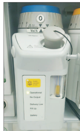
Fig. 1. The yellow discoloration of desflurane observed through the vaporizer window.
