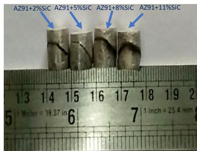
**Figure 10.** Fractured samples in a compression test.
