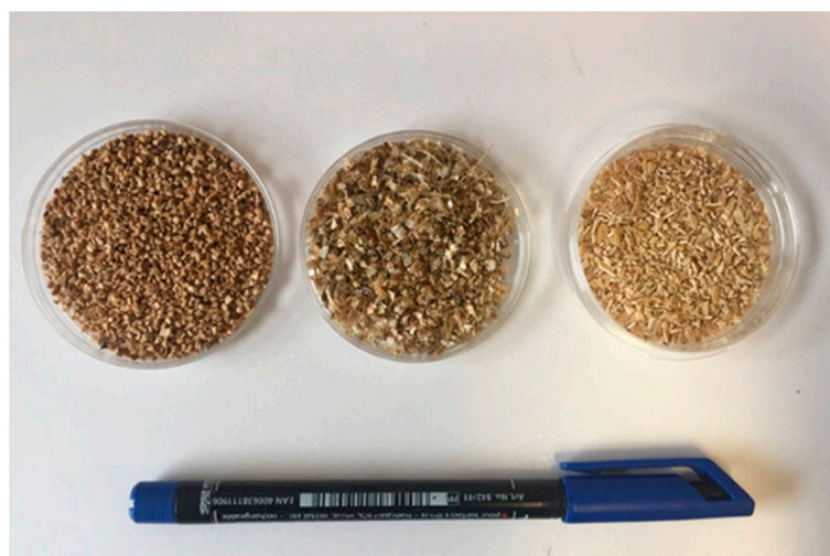
Figure 1. Sieved fraction (between 1 and 2 mm) of biosorbents (left to right: hazelnut, pistachio, walnut).
