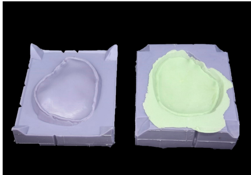
Figure 5. Molded patient-specific polymethylmethacrylate cranial implant with excess material.
