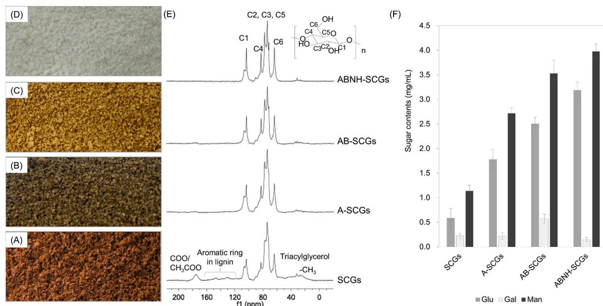
**Fig. 2.** Visual appearance of (A) raw spent coffee grounds (SCGs), (B) alkali-pretreated SCGs (A-SCGs), (C) bleached A-SCGs (AB-SCGs), and (D) NaOH-hydrogen peroxide-pretreated (ABNH-SCGs). (E) Solid-state  $^{13}\text{C}$ -nuclear magnetic resonance (NMR) spectra of untreated and pretreated SCGs. (F) Enzymatic hydrolysis of raw and pretreated SCGs using in house-produced cellulase and mannanase (Glu, glucose; Gal, galactose; and Man, mannose).
