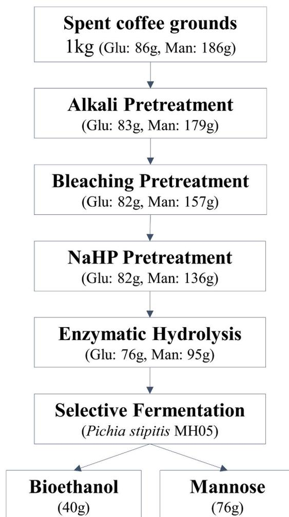
Fig. 5. Overall mass balance for the production of mannose and bioethanol from SCG.
