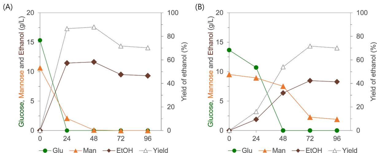
Fig. 4. The fermentation profiles for SCG hydrolysates using (A) parental *P. stipitis* strain YN14 and (B) mutant *P. stipitis* strain MH05 (Glu, Glucose; Man, mannose; EtOH, ethanol).
