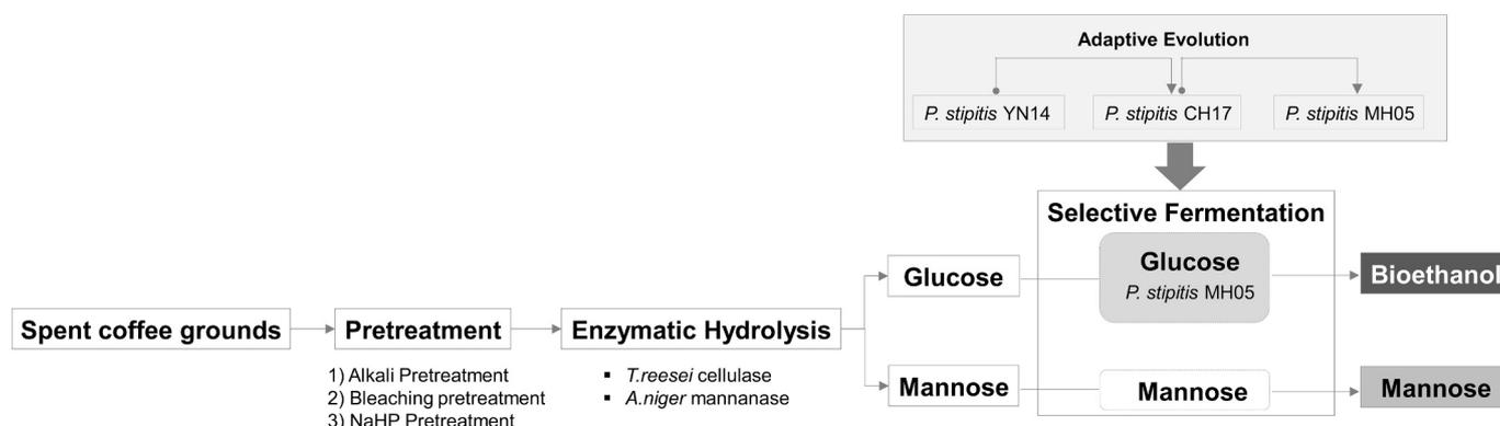
Fig. 1. Production process of D-mannose and bioethanol from SCGs.
