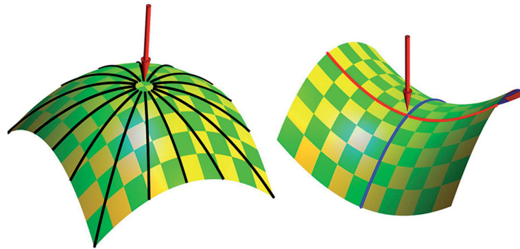
Figure A3. Examples of surface irradiance flow. The direction of the uniform, unidirectional irradiating beam is indicated with red arrows. At left, a convexity on which one obtains a divergent flow. At right, a saddle on which one obtains a deformation flow. Along the red curve, the flow approaches the center, along the blue curve, it moves away from the center.
