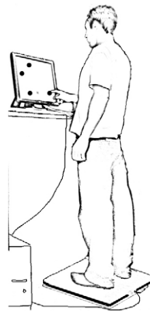
Figure 1. The experiment setup. The participant was instructed to stand on the forceplate in a quiet stance position, in front of the touch screen. The forceplate's output data was streamed into the same desktop PC that presented and controlled the touch sequence task. doi:10.1371/journal.pone.0043488.g001
