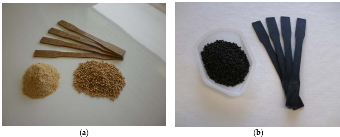
Figure 1. Images of HDPE composite pellets and tensile samples from untreated wood (a, wood polymer composites, WPC) and biochar (b, Biochar polymer composites, BPC).
