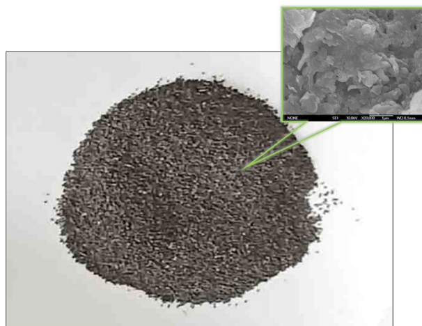
Figure 2. Photograph and SEM image of scoria.
