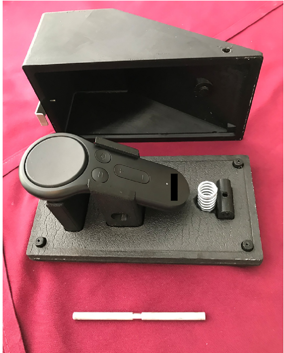
Fig 2. Remote controller inside foot pedal.
