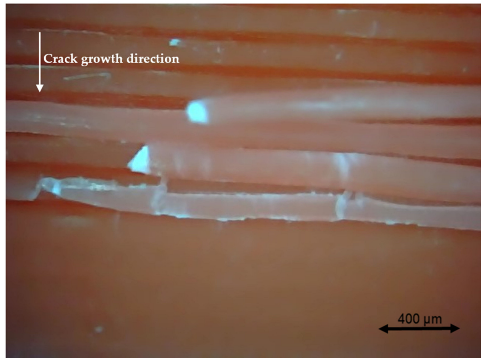
Figure 21. Specimen with a nozzle size of 0.8 mm, Y building orientation, and layer thickness of 0.15 mm.
