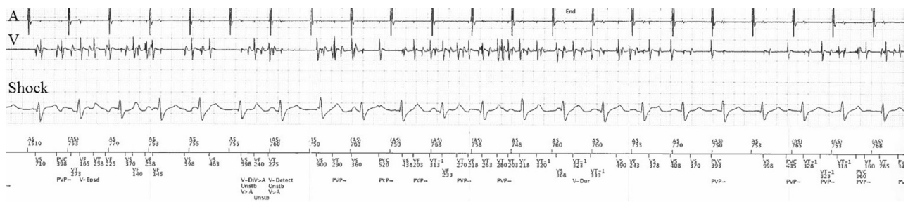
Figure 2 Electrograms (EGMs) showing electromagnetic interference (EMI) that was sensed as ventricular tachycardia / ventricular fibrillation but not treated owing to presence of a magnet. A = right atrial lead EGMs, true bipolar sensing; V = right ventricular (RV) lead EGMs, integrated-bipolar sensing from the tip electrode to the RV coil; Shock = “shock” EGM, a far-field signal recorded from the pulse generator to the RV coil. Again, note the only very subtle noise on the shock EGM, in contrast to the large-amplitude EMI seen on the RV EGM.
