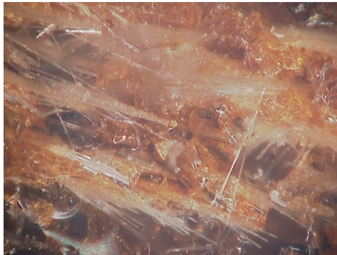
Figure 10. The fracture surface of 30 wt.% GF/p-DCPD composite.
