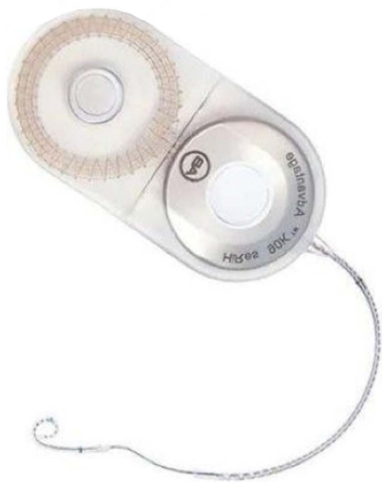
Fig 3. Physical structure of the cochlear implant.
