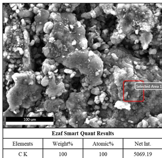
**Figure 2.** Surface morphology of MWCNT-NP utilizing SEM analysis.
