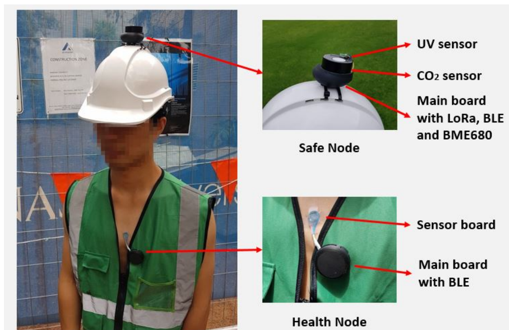
Figure 3. The Safe Node and Health Node are attached to the subject' helmet and body.
