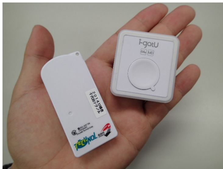
Fig 2. The “D-shuttle” (left) personal dosimeter and “i-gotU” (right) GPS receiver used in this study.
