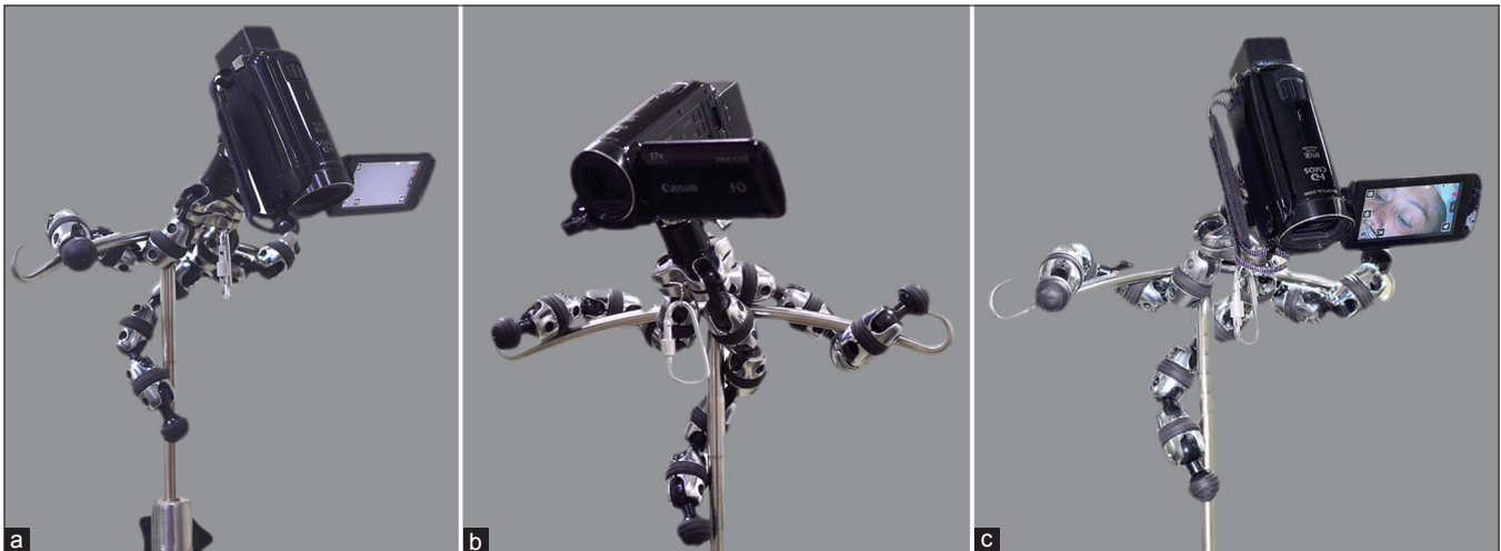
Figure 2: A camcorder fixed on the Gorillapod® with its legs wrapped around the IV stand at the top – over the horizontal bar with hooks for hanging IV fluid bags (a). The IV fluid stand is at the head-end of the patient on the side opposite to the eye being operated. The position, angulation and the focal length of the camera is adjusted such that the area of interest is captured (b and c)
