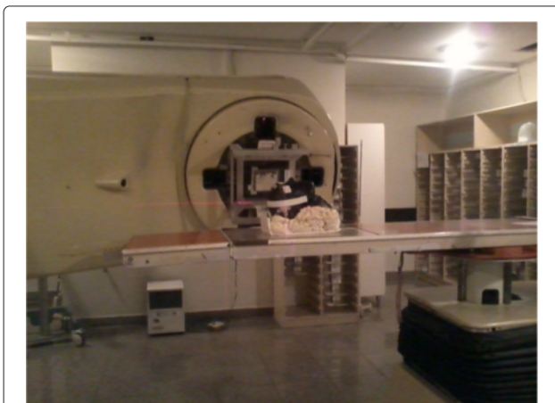
Figure 3 Phantom positioning in relation to the accelerator gantry. Planning and beam positioning indicated, based on the CT images.
