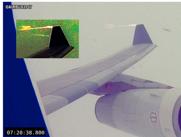
Figure 8. The image of the static discharge on the left wing. Color-adjacent inset is shown to enhance the visual perception. The discharge follows the vortex channel core of reduced pressure. The time is indicated in the left corner and corresponds to TR4.
