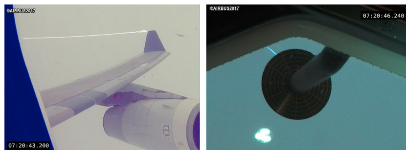
Figure 9. The original camera images of the discharge activity from the aircraft. Left image shows the vortex channel re-brightening behind the left wing tip. Right image shows the probe for ice accretion measurement located on the cockpit left top. Both images contain discharges that happened synchronously with gamma ray enhancements.
