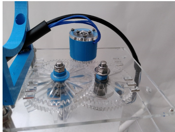
Figure 6. The reducer based on four cogwheels, a drive wheel ( bottom left ), and a Maltese cross ( bottom right ).
