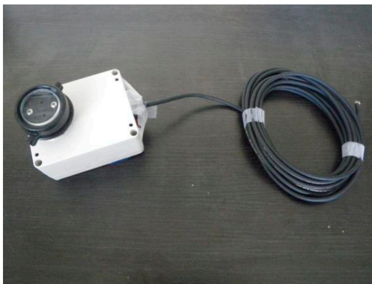
Figure 2. Sensor housing. A cable was used to power the instruments while a wireless link was used for communicating data.
