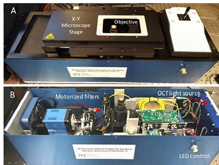
Fig 5. Photograph of the multimodal microscope. A. General view; B- Inside view.
