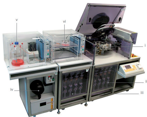
Figure 1. Borgwaldt RM20S smoking machine. (i) Cigarette smoke generator. (ii) Original four-syringe system. (iii) Four-syringe extension. (iv) Air-flow controller. (v) Cell culture media maintained at 37 °C. (vi) British American Tobacco's exposure chamber housed at 37 °C, attached to the smoke diluter and culture media (modified from Adamson et al., 2011).
