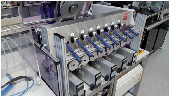
Figure 3. Vype ePen e-cigarettes are attached to the adapted Borgwaldt RM20S by bypassing the cigarette smoke generator.
