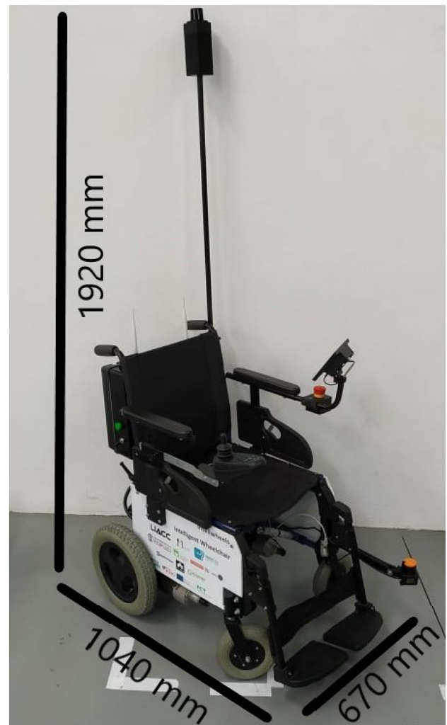
Fig. 3 Final appearance of the wheelchair with an indication of its dimensions
