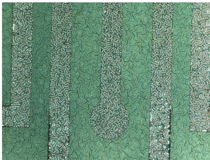
Figure A1. Cr/Au/Cr metal layer deposited on PDMS. Conductive tracks were designed to be 100 \mu\text{m} in width and the circular electrode to be 200 \mu\text{m} in diameter.
