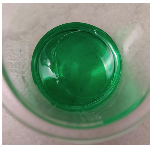
Figure 5. Polymer film immersed in nitric(V) acid solution.
