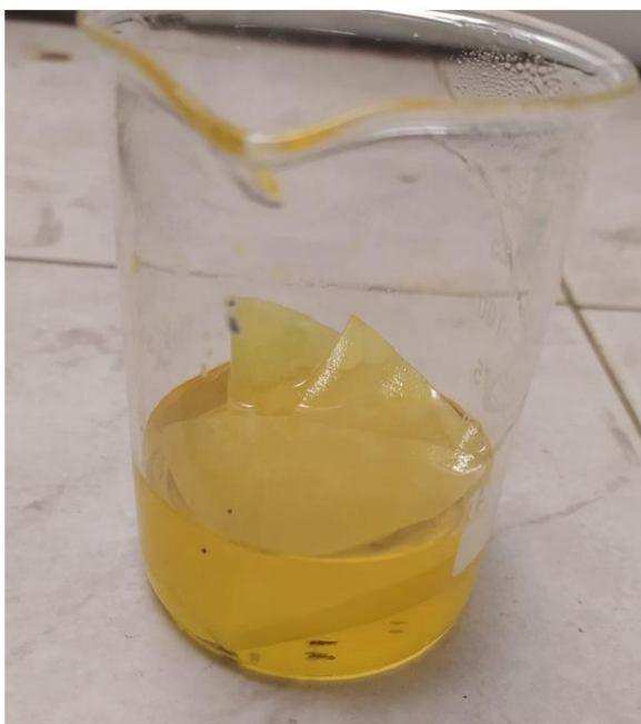
Figure 4. Preparation of computer pin samples for analysis: (a) computer pins dissolved in nitric (V) acid—gold flakes visible on the surface; (b) computer pins dissolved in nitric (V) acid—visible undissolved pin residues; (c)—dissolving of insoluble components in nitric (V) acid residue of computer pins in aqua regia.
