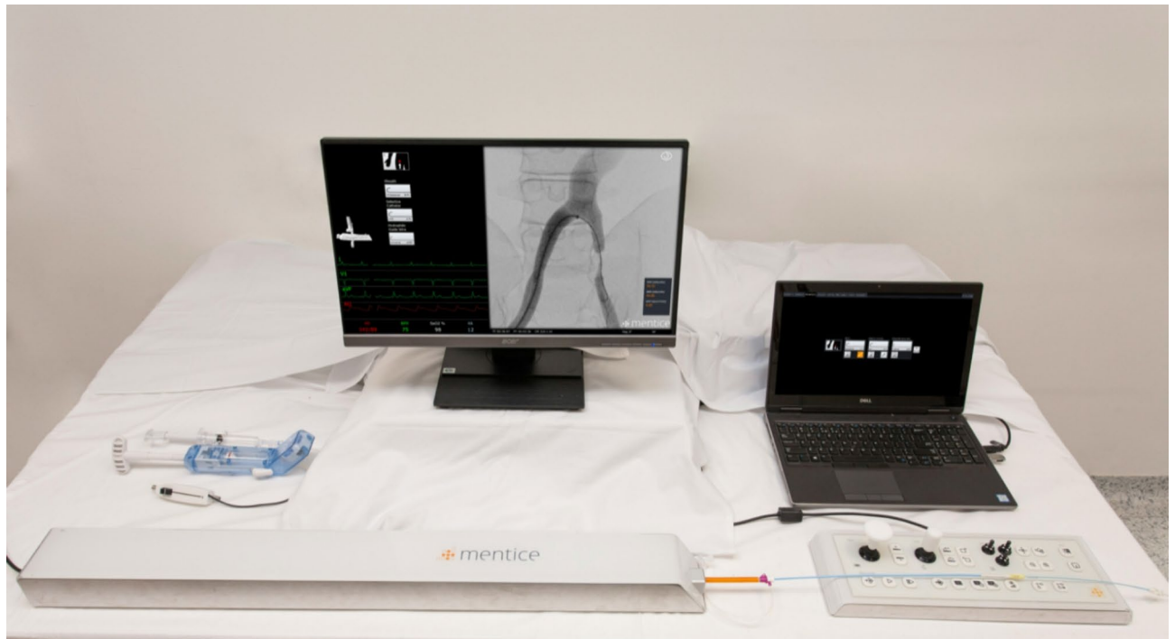
Fig. 2. Experimental setup for the simulator training sessions, including the VIST G5 Mentece endovascular simulator, control joysticks, 3D monitor, fluoroscopy, CINE pedals, and device insertion model. This figure illustrates the comprehensive simulation environment used to emulate a catheter lab, enhancing the training experience for the participants.
