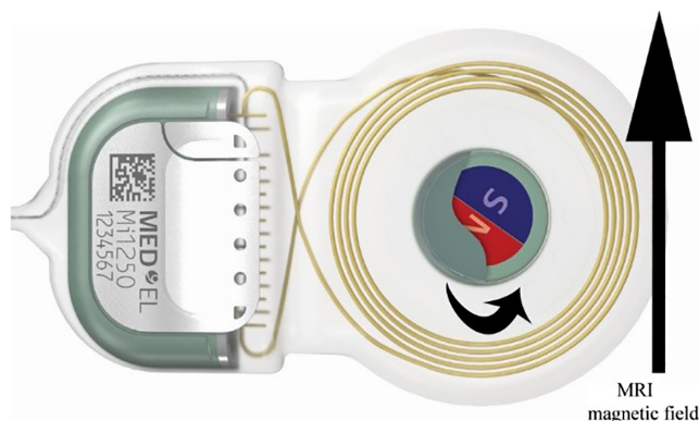
Fig. 1. Diametric magnet poles rotate within the device to align with the static magnetic field of the magnetic resonance scanner. MRI = magnetic resonance imaging.
