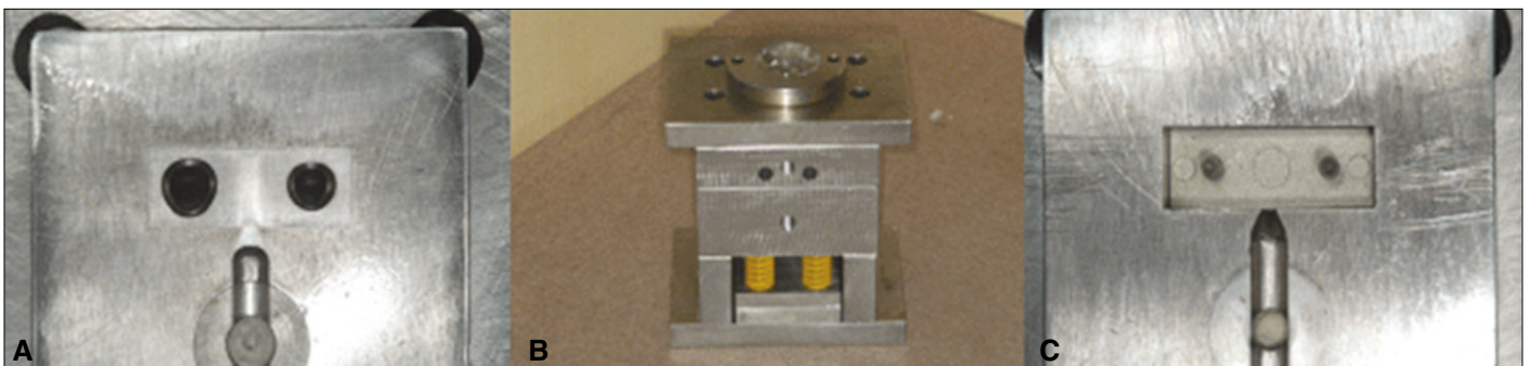
Fig. 2. Fabricated injection mold. A: Abutment part of mold, B: Assembled mold, C: Base part of mold.
