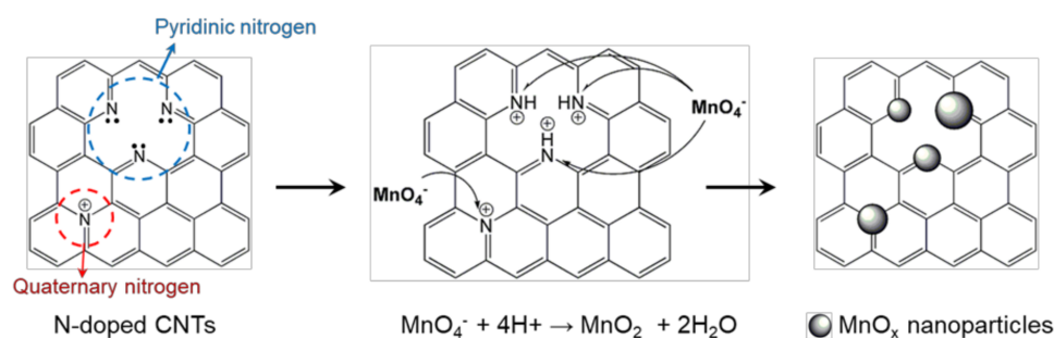
Figure 4. Schematic diagram of possible nucleation mechanism of \text{MnO}_x nanoparticles at quaternary N ( \text{N}_Q ) and pyridinic N ( \text{N}_P ).
