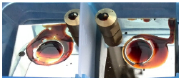
Figure 4. Photographic image of composite films after Pr irradiation and friction test.
