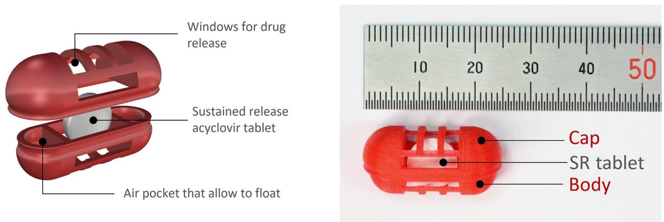
**Fig 1. The structure of the gastroretentive (GR) system.** The novel GR system composed of the 3D printed gastro-floating device and acyclovir sustained-release (SR) tablet inside the device.
